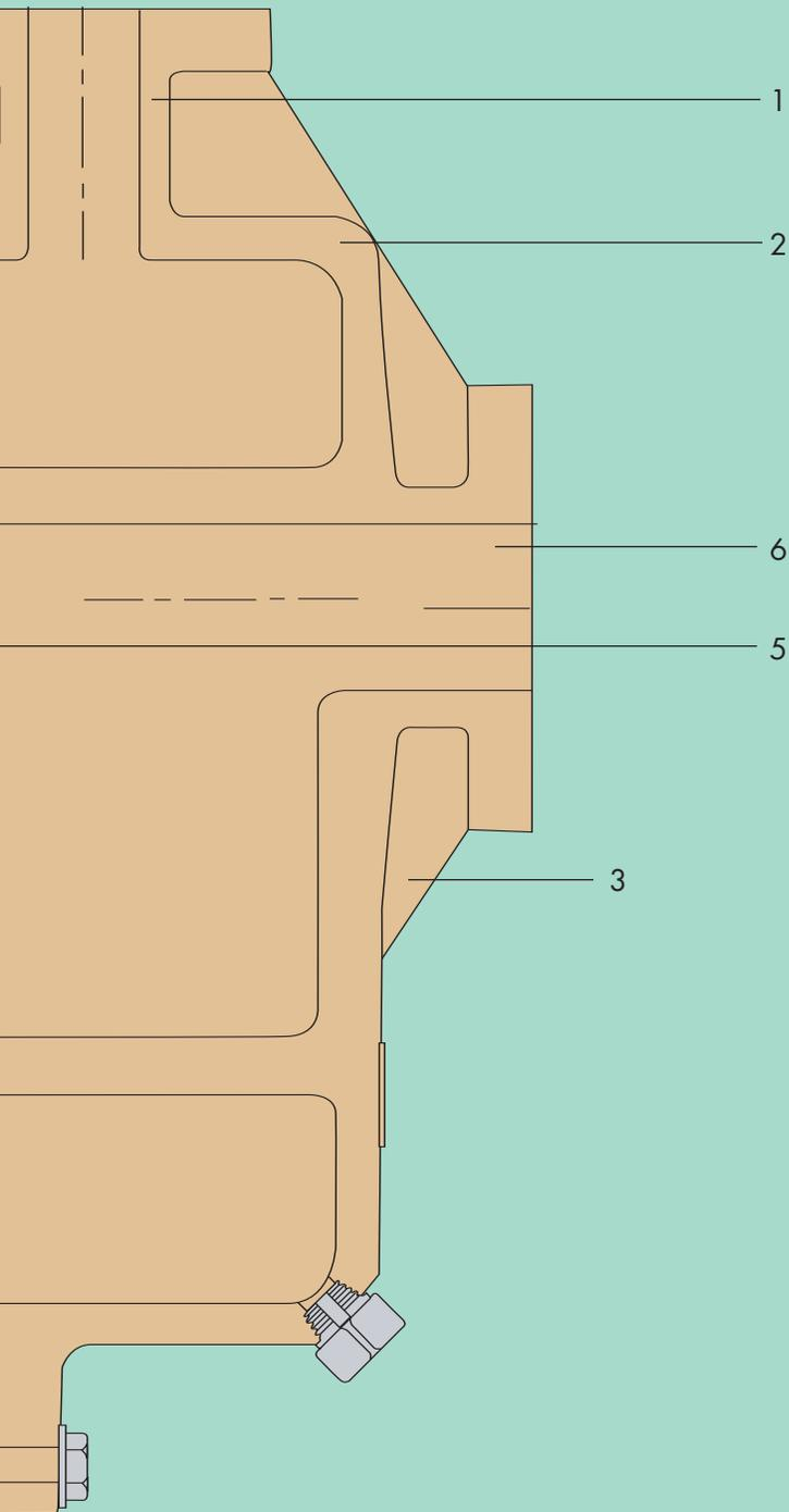
1. **FIBERGLASS CONSTRUCTION** of all wetted parts in vinyl ester resin provides tough corrosion-resistance for a wide range of difficult liquids.
